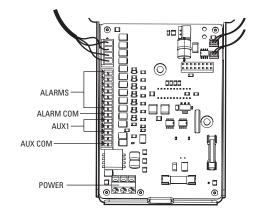
Connect a 10/100/1000BaseT network Cat5e (or better) cable to the RJ-45 network connector located inside the back box. Check the LED indicators located inside the back box to check unit status, network status, and network activity.
